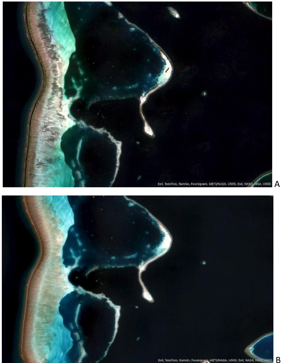
Figure 17 - Original processed image from 2017 of Corals in the Maldives (A); Radiometrically Normalised image from 2024 of Corals in the Maldives (B).
